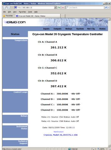
**Utility Software:** Utility software is provided that connects any Windows based personal computer to the Model 26 via any of its remote interfaces. This software provides a graphical control panel that greatly simplifies instrument setup and configuration. Features include:
