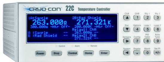
The model 22C is a two-input, four-control loop cryogenic temperature controller capable of operation to <math><200\text{mK}</math>. While enhanced for ultra-low temperature operation, a wide variety of general purpose sensors and heaters are also supported.
