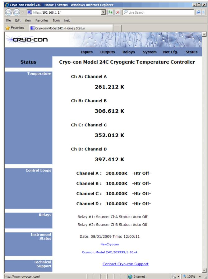
**Utility Software:** Utility software is provided that connects any Windows based personal computer to the Model 22C via any of its remote interfaces. This software provides a graphical control panel that greatly simplifies instrument setup and configuration. Features include:
